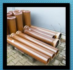
Vitrified clay pipe is made from a clay – shale blend that has been subjected to a high temperature. This vitrification results in a hard, firm ceramic. A salt glazing is applied to the pipe's interior and exterior surfaces.
